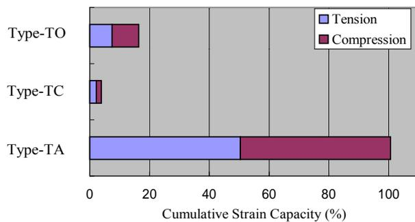
Figure 16 Cumulative Equivalent Strain Capacity until Fracture
