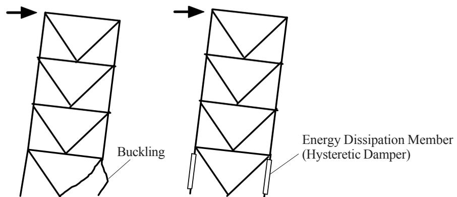
Figure 1. Damage Tolerant Concept for Truss Frame
