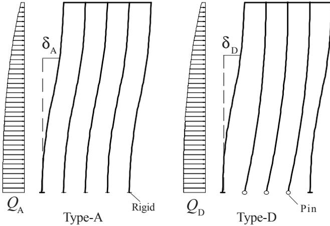
Figure 5 Models for Stiffness Evaluation
