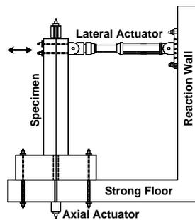
Figure 1. Test setup
