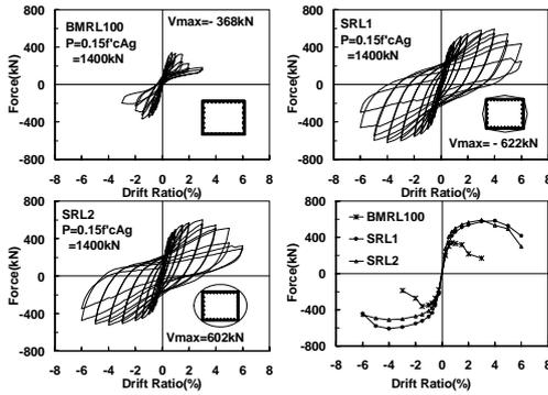
Figure 5. Cyclic lateral load vs. deflection relationships
