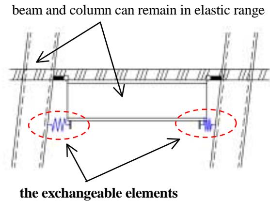
Fig. 4 The desirable deformation
