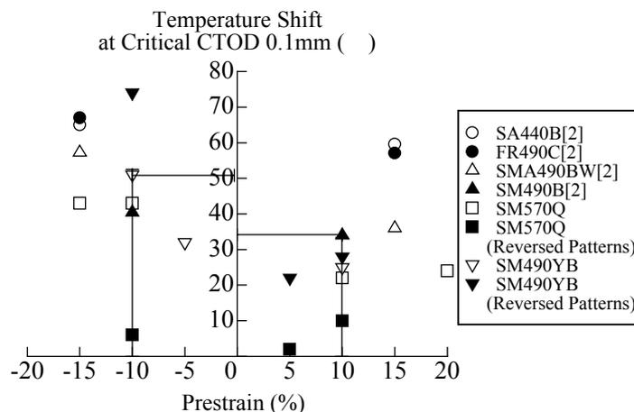
Figure 12 Relationship between Prestrain and Temperature Shift of CTOD Curves
