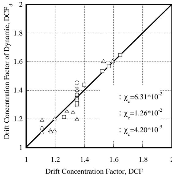
Figure 8 Comparison between dynamic  $DCF_d$  and static DCF
