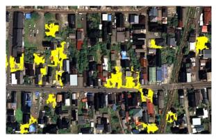
Figure 12. The result of extracted debris after subtraction of the pre-event debris areas and applying the minimum area filter ( $A_{min}$ =58m<sup>2</sup>).
