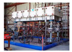
Fig. 1 Shaking Test specimen of simple supported bridge with different substructure stiffness
