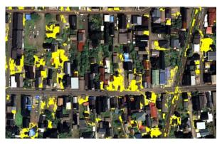
Figure 10. The result of extracted debris by the object-based level-slice method. Many small commission errors are seen.
