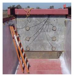
Figure 2: Abutment backwall section suspended above seat box
