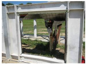
Figure 7. SPSW 2 After Test 2
