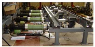
Figure 1. The multiple support excitation test bed.
