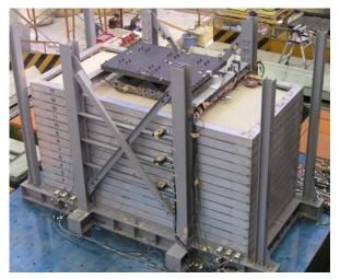
Photograph 1 Model of Soil-pile-structure system (S-S Model)
