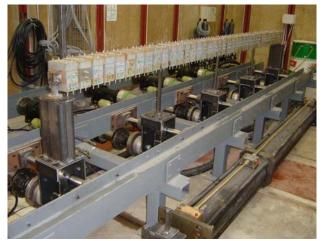
Figure 3. The LLL viaduct bridge on the test bed.
