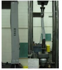
Photo 1 Local Buckling Failure
