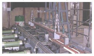
Figure 4. A cable stay bridge model on the test bed.
