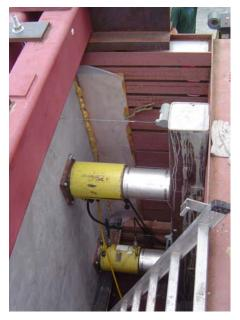
Figure 3: Loading mechanism behind backwall
