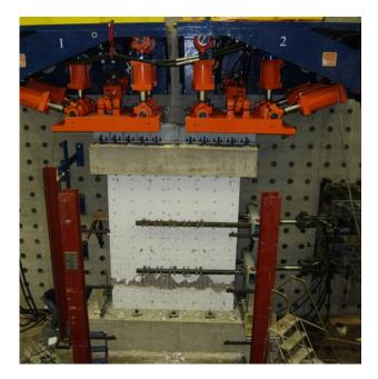
Figure 3 Planar Wall Test Specimen Following Testing to a Maximum Drift of 1.5% at NEES@UIUC
