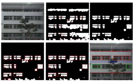
Figure 5: Automatic identification of mirroring axis and region for self-mending occlusions. From upper left to lower right: (a) original; (b) region growing; (c) area histogram filtering; (d) homogeneity test; (e) location filtering; (f) identified mirroring axis and region.
