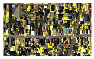
Figure 11. The result obtained by applying the debris extraction procedure to the pre-event digital image.
