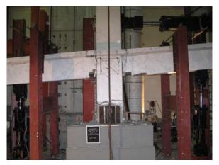
Figure 10 Overall specimen at final cycle to drift ratio  $\gamma = 7\%$
