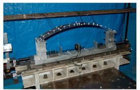
Photograph 1 Experimental Device of Arch Structure (Fa model)
