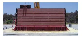
Figure 1: Soil container on shake table
