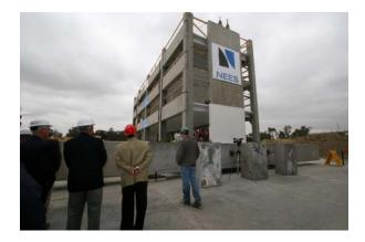
Figure 2 Half Scale Precast Structure Ready for Test on NEES@UCSD Shake Table
