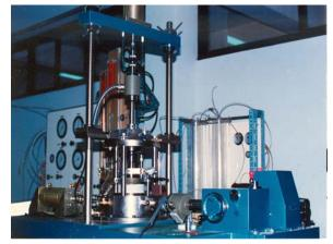
Figure 1 Simple shear Apparatus
