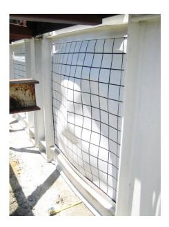
Figure 6. Backside of SPSW 1 After Test 1
